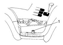
Check the brake fluid level frequently for the auxiliary brake system. The reservoir is located under the seat or near the foot brake. Maintain the fluid level between the maximum and minimum marks.
